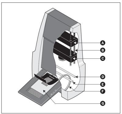
Figure 3: Cut-away view of Flextight 848
