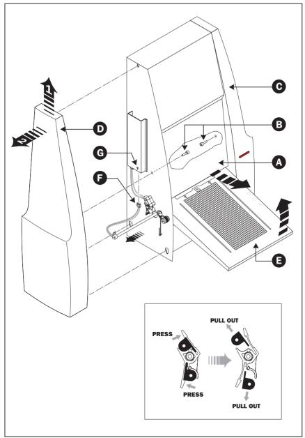
Figure 7: Replacing the Light Tubes
