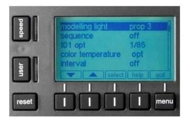
The desired unit functions are selected with the keys " $\nabla/\blacktriangle$ " and confirmed with the key "select". The selected function is visually highlighted with a bar.
